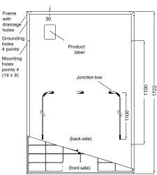
Note: dimensions in mm, tolerance +/- 2 mm
